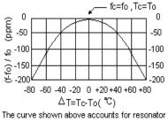
contribution only and does not include LC component temperature characteristics.
